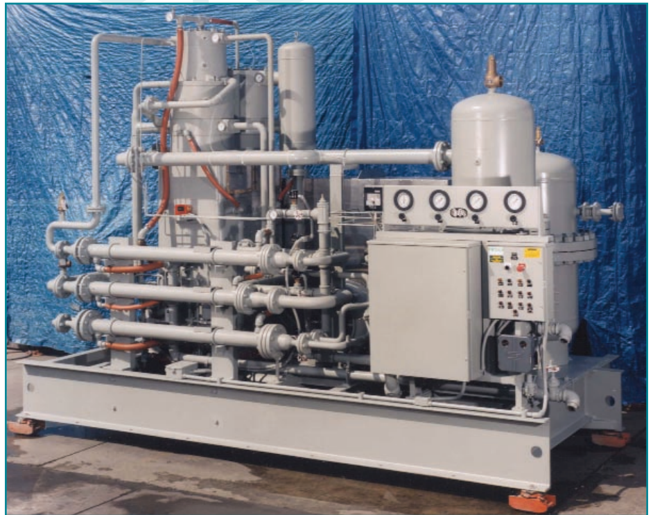
This 350 HP RIX compressor is boosting oxygen to 220 psig for a steel plant in the U.S.
