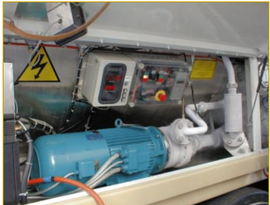
An ACD CRYO laser tank filling centrifugal pump system with a variable frequency drive installed on a cryogenic container.
