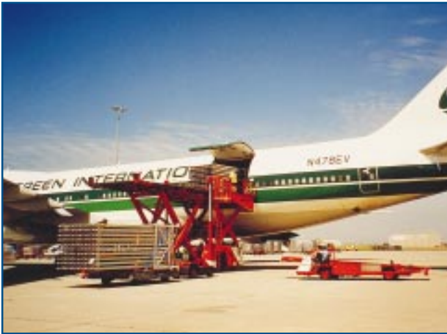
The IWI Cryoquip vaporizers are secured in the hull of a 747 using only partial pallets for support at the heavier end of the units.
