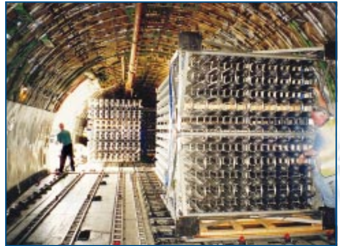
Eight ambient air vaporizers are loaded onto an Evergreen 747 charter bound for Indonesia.
