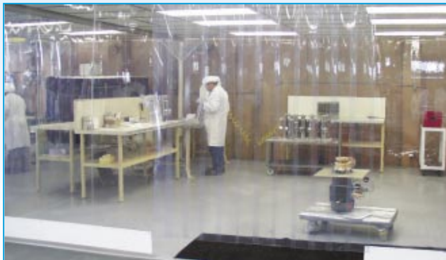
The 600 ft 2 (56 m 2 ) clean room has two separate areas that vary from class 100 to class 10,000 standards.
