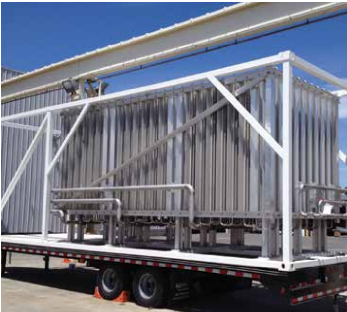
Figure 4 – Ambient with three circuits in one frame
