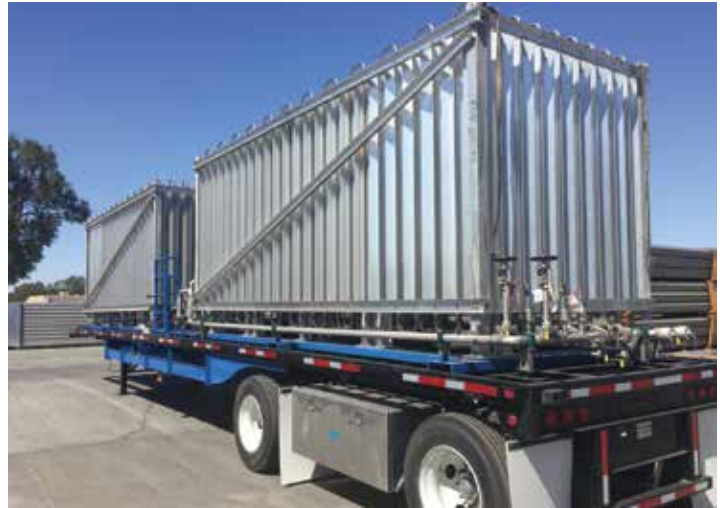
Figure 1- Trailer mounted natural draft ambient system
