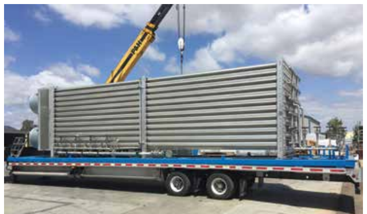
Figure 3 - Horizontal fan ambient vaporizer
